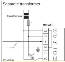
Terminal assignment for controller with 3-wire connection
